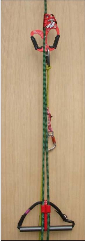
**Figure 5. If a climber prefers the angled grip of the Kong Twin and still wants to use the lower Mar-Bar for his or her feet, the upper Mar-Bar can be easily exchanged for the Twin. Some type of backup system is recommended. Here the tether attached to the Twin is a Prusik loop with a webbing sling as an adjuster.**
