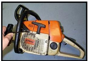
If your saw has compacted sawdust or dirt present near air intake areas, the amount of cooling air allowed to flow across the cylinder will be limited and may contribute to overheating of the engine and piston seizure.
