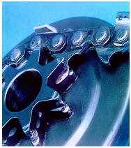
If the sprocket is worn past its normal use it will cause vibration and premature chain wear. Wear patterns greater than twenty thousands would indicate its time to change the sprocket.
