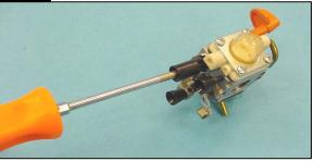
Improper field adjustments made to carburetors can lead to other issues and failures. Factory settings are important to maintain while the saw is in the field due to internal jet and port sizing as well as emissions considerations. Improperly set carburetors can lead to lean fuel-air ratios, resulting in lack of engine lubrication and ultimately premature failure. If there is a concern of carburetor contamination or adjustment take the unit to a qualified service technician.
