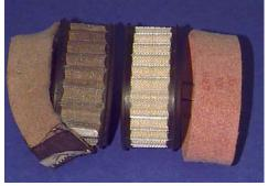
A dirty air filter can contribute to bogging the unit down and poor performance. Dirt left on air filters can also cause dirt ingestion. Dirt in the engine will lead to premature piston, rings, seals, and bearing failure. Air filter maintenance and periodic replacement is very important.
