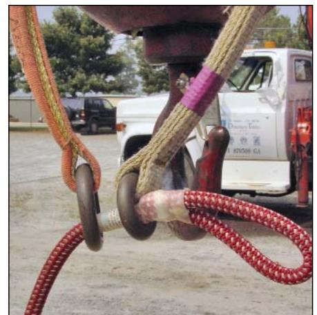
**Fig. D:** The climbing line is threaded through the big ring first, then through the small ring—this is the opposite of the way that the rope is threaded when a false crotch is used in a tree.
