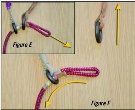
rope is installed (Fig. E), then the rope will exit through the big ring first, then through the small ring when the rope is retrieved. If the rope catches on the small ring (Fig. F) the rope could pull the false crotch up to
