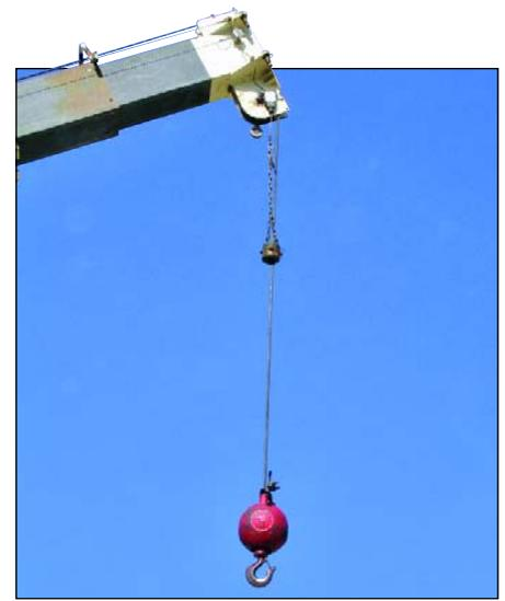
**Fig. A:** According to ANSI Z133.1-2006, a qualified arborist may tie-in to the crane’s boom or load line (cable), but not the hook. (State, regional, or local regulations may be different, e.g. Cal-OSHA requires that the tree worker be secured to an independent line attached above the crane’s hook and be “...secured to a crane’s hook that shall be closed with a positive locking device”.)
