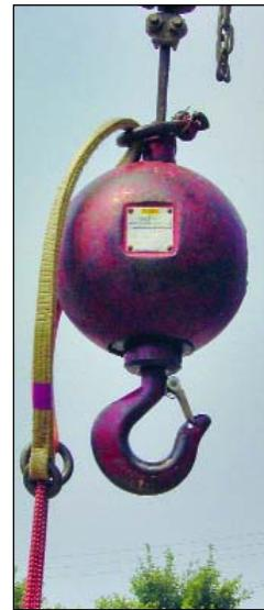
**Fig. C:** ...and place a false crotch through the shackle.
