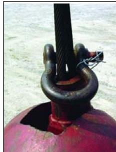
**Fig. B:** One option to attach the climber to the crane is to place a shackle on the cable above the ball, secure the pin of the shackle with a piece of sturdy, weather-proof wire ...
