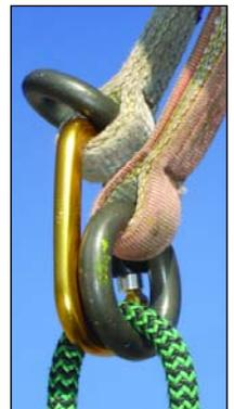
**Figure H -** *The climbing line is threaded only through the big ring and the carabiner (not through the small ring). Because the carabiner has a large opening the rope may go through either the big ring first or through the carabiner first.*
